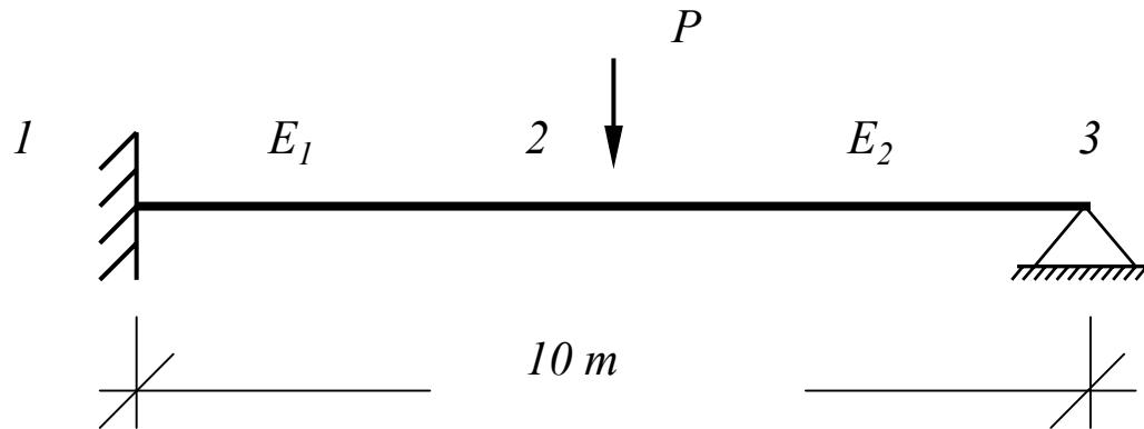
$$A = 0.086 \text{ } m^2 \quad I = 10^{-4} \text{ } m^4 \quad E \text{ (nominal)} = 200 \text{ } GPa$$
