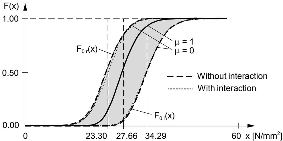
Figure 14. Fuzzy probability distribution function  $\tilde{F}(x)$  with and without consideration of interaction between  $\tilde{m}_x$ ,  $\tilde{\sigma}_x$  and  $\tilde{a}$ ; probability distribution functions  $F_{0l}(x)$  and  $F_{0r}(x)$
