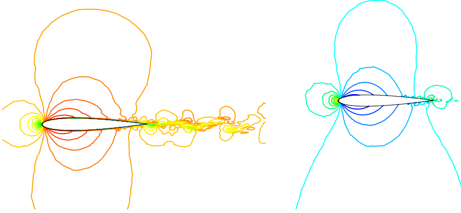
Figure 2. The fluid velocity and pressure isolines for inlet velocity U = 25 \text{ m s}^{-1}
