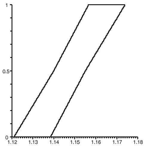
ullet P-box enclosure (using SIR with 100 partitions) of variable  $x_1$  at time t=10
