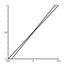
ullet P-box enclosure of variable  $x_1$  at time t=10 computed with Risk Calc, using Taylor model from VSPODE
