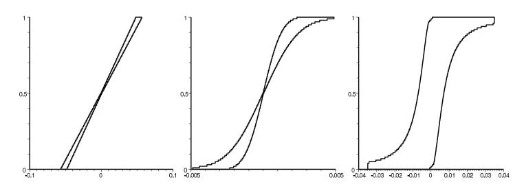
ullet P-box enclosure of variable  $x_1$  at t=10 computed with Risk Calc using Taylor model from VSPODE
