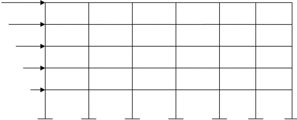
**Figure 3.3. Earthquake/Wind Load (Static Equivalent) presence on a portal frame**
