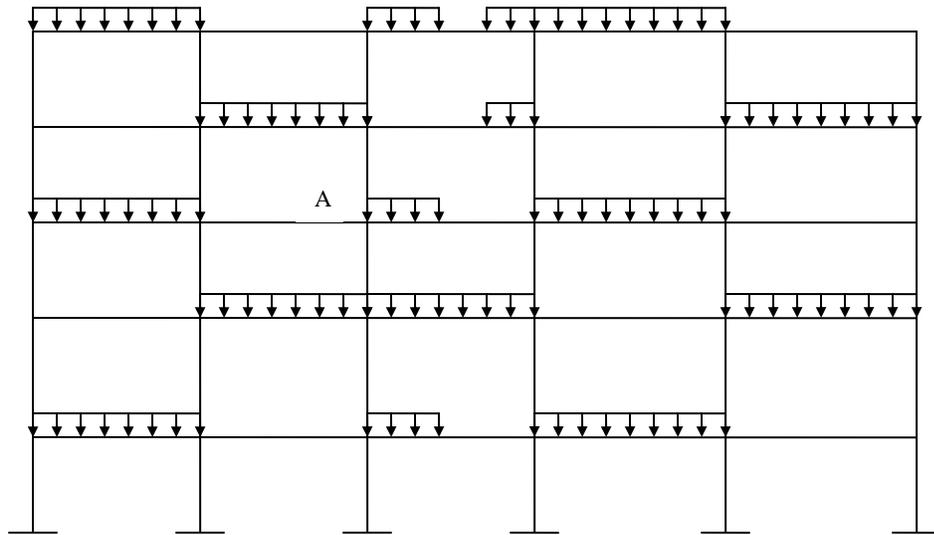
**Figure 2.4b. Live load pattern for negative moment at section A**
