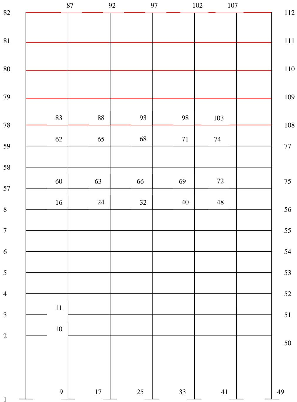
**Figure 10.1. Joints numbering for fifteen-floor portal frame**
