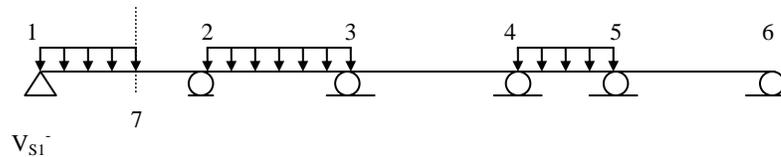
**Figure 1.8b. Load pattern for maximum negative shear at 7**
