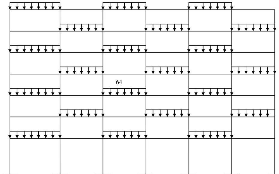
Figure 7.1. Case 1: Live load pattern for maximum span moments in beam
