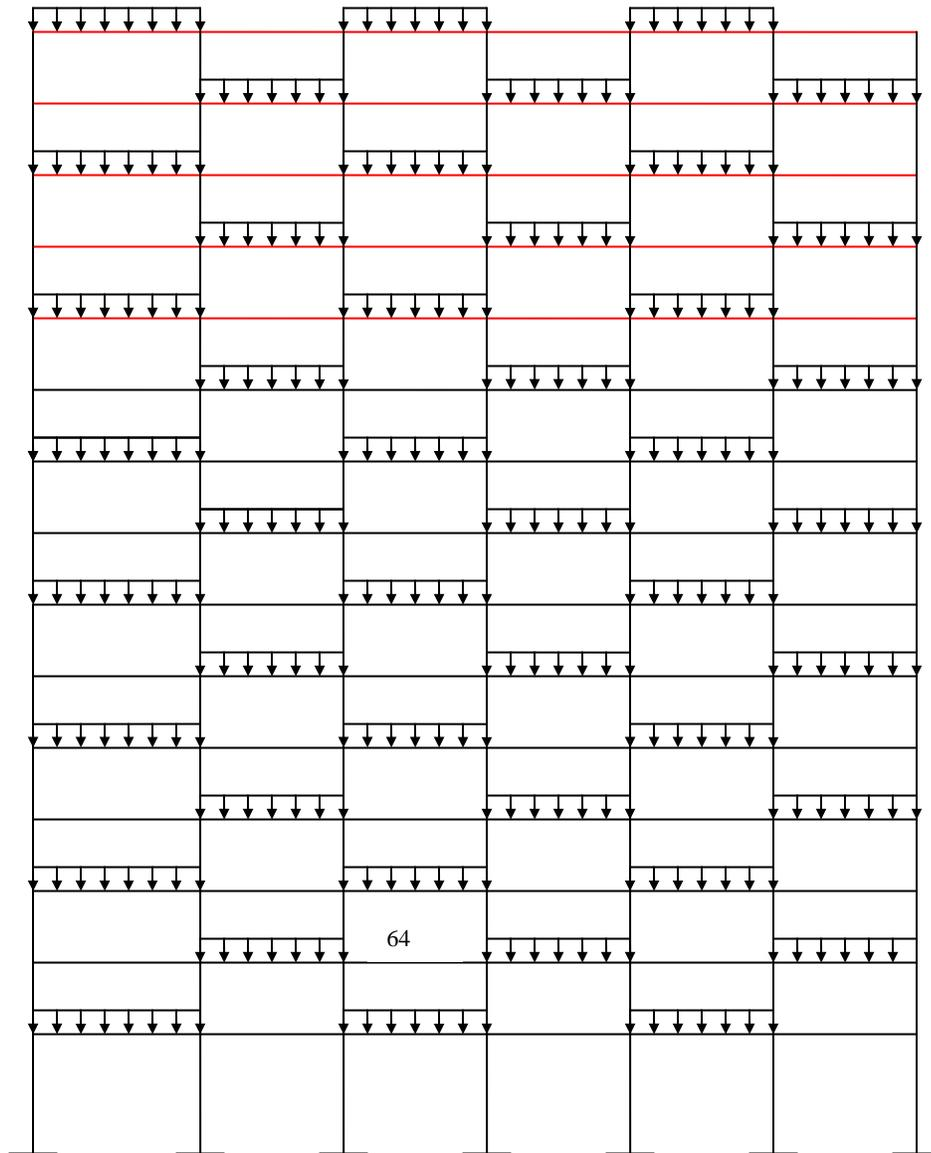
**Figure 11.1. Case 1: live load pattern for maximum span moment in beam– fifteen-floor frame**
