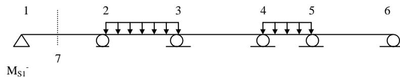
**Figure 1.10b. Load pattern for maximum negative moment at 7**
