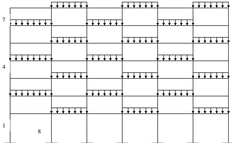
**Figure 7.5. Case 3: Live load pattern C for maximum/minimum end moment in a column**
