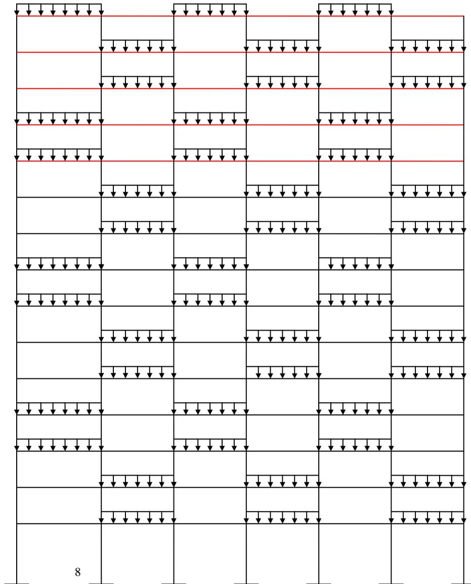
**Figure 11.4. Case 3: Live load pattern B for maximum/minimum end moment in column– fifteen-floor frame**
