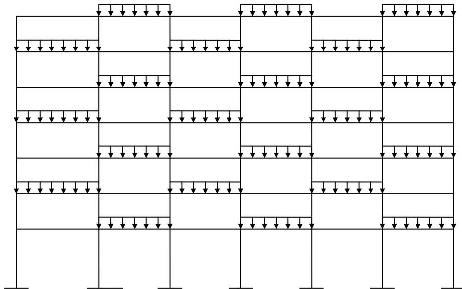
**Figure 3.2. Live load presence on a portal frame (checker-board pattern)**
