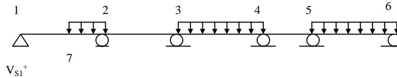
**Figure 1.7b. Load pattern for maximum positive shear at 7**
