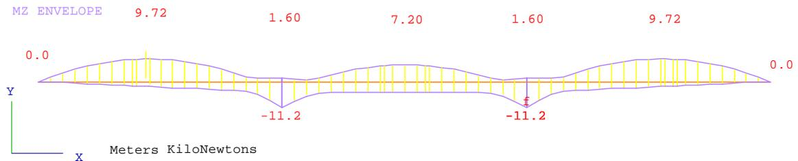
**Figure 4.1b. Moment envelope for all possible live load patterns (GTSTRUDL)**
