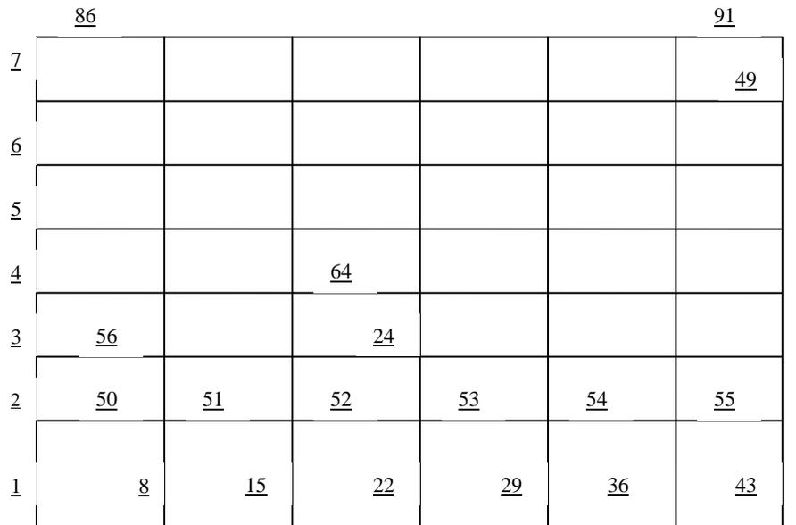
**Figure 6.4. Frame elements numbering for seven-floor frame**
