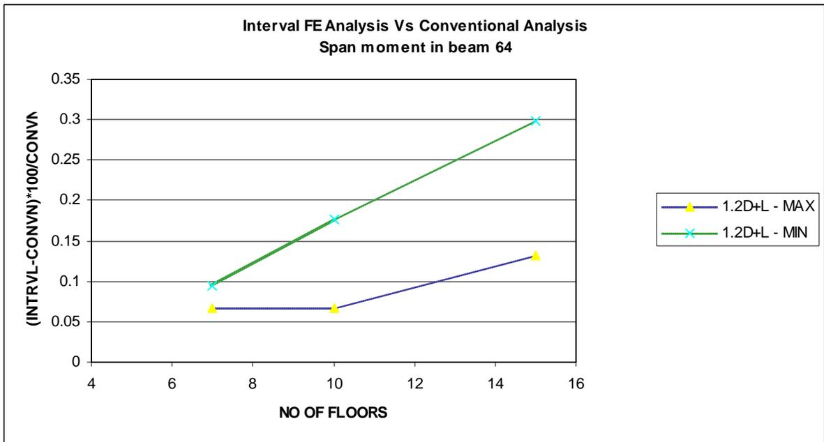
**Figure 12b. Maximum and Minimum Span Moment in Beam 64 - Percentage deviation Vs number of floor for load combination 1.2 D + L**
