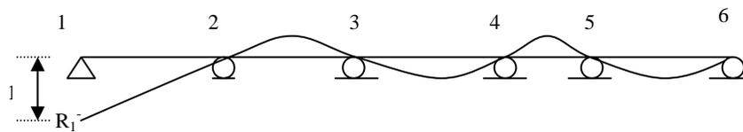
**Figure 1.2a. Influence Line for negative reaction at support 1**
