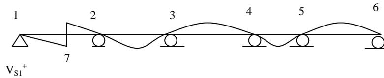
**Figure 1.7a. Influence line for positive shear at 7**
