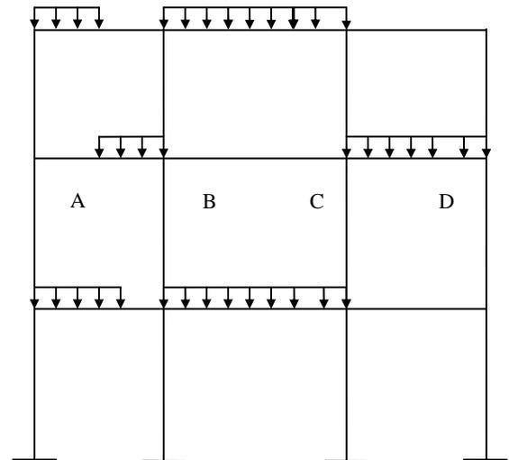
**Figure 2.1b. Load Pattern for maximum positive shear at mid-span of AB**
