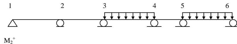
**Figure 1.4b. Load pattern for maximum positive moment at support 2**
