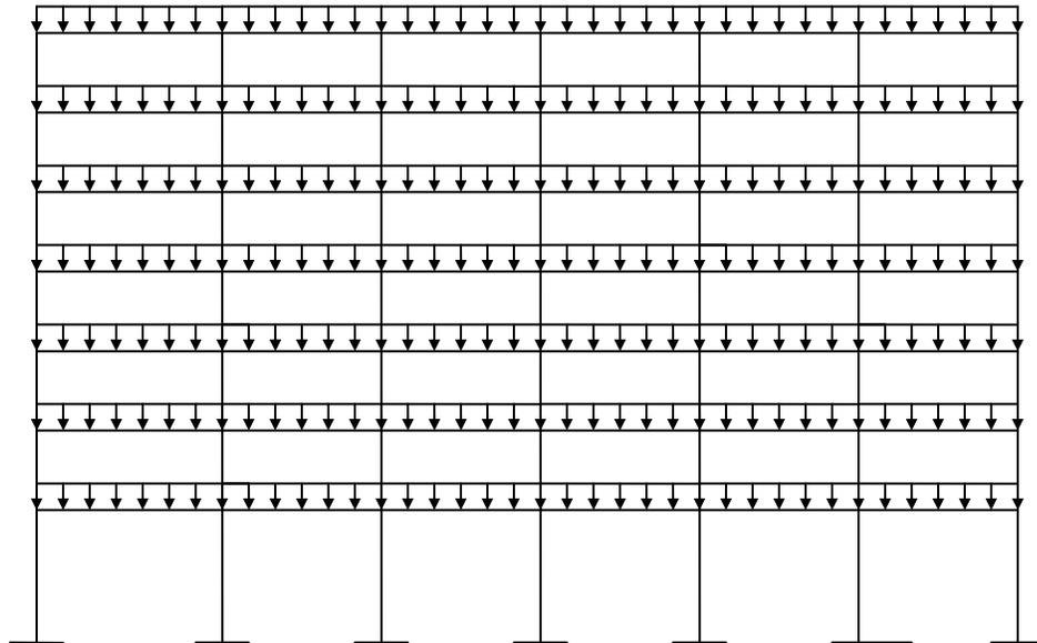
**Figure 3.1. Dead Load Presence on a Portal Frame**
