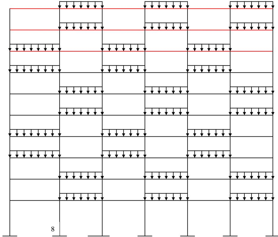
**Figure 9.4. Case 3: Live load pattern B for end moment at the end of column– ten floors frame**
