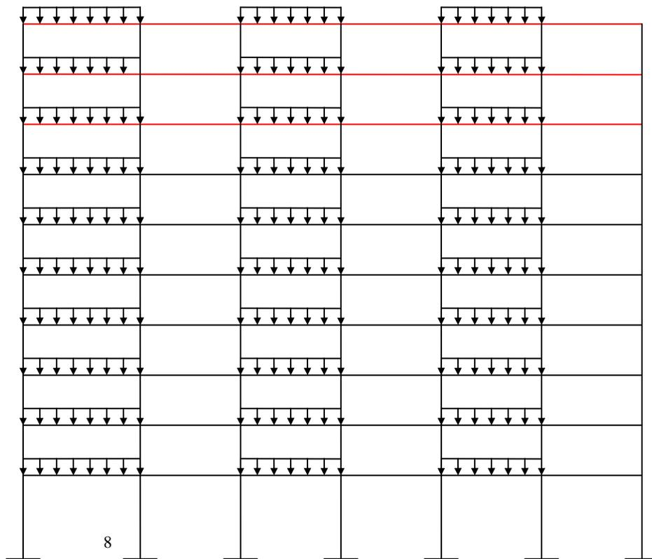
Figure 9.3. Case 3: Live load pattern A for end moment at the end of column element – ten floors frame
