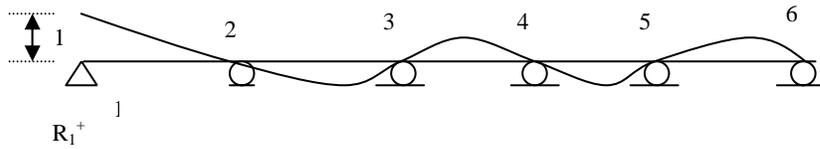
**Figure 1.1a. Influence Line for positive reaction at support 1**
