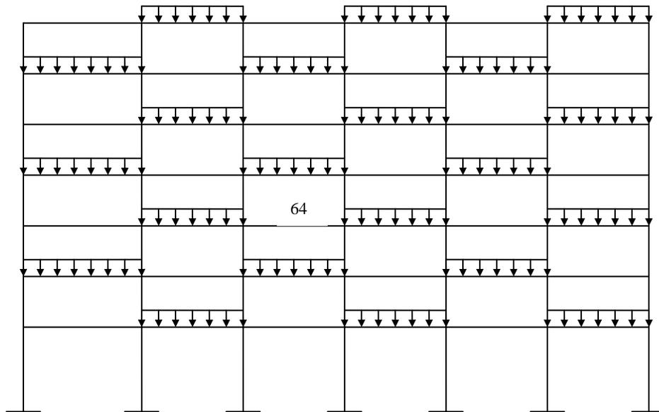
**Figure 7.2. Case 2: Live load pattern for minimum span moment in beam**
