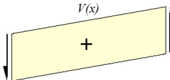
**Figure 1.6. Sign convention for positive shear**
