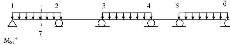
**Figure 1.9b. Load pattern for maximum positive moment at 7**
