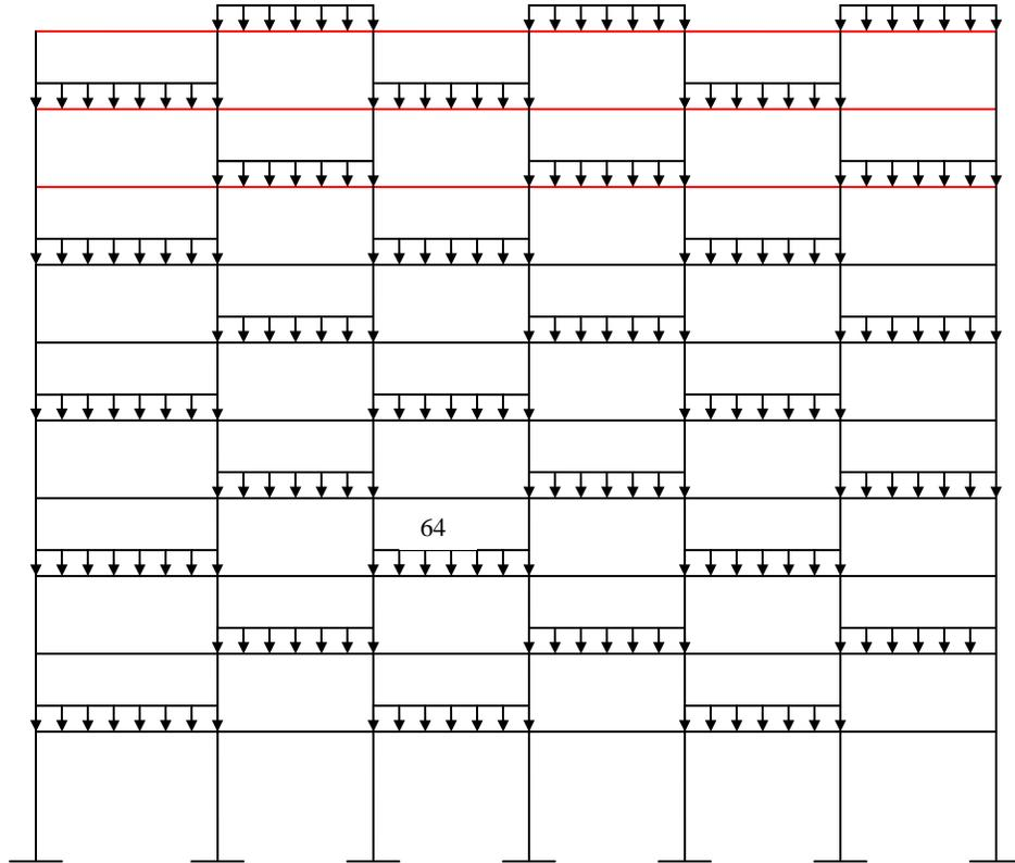
**Figure 9.1. Case 1: Live load pattern for maximum span moment in beam – ten floors frame**
