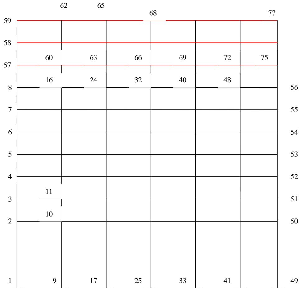
**Figure 8.1. Joints numbering for ten floors frame**
