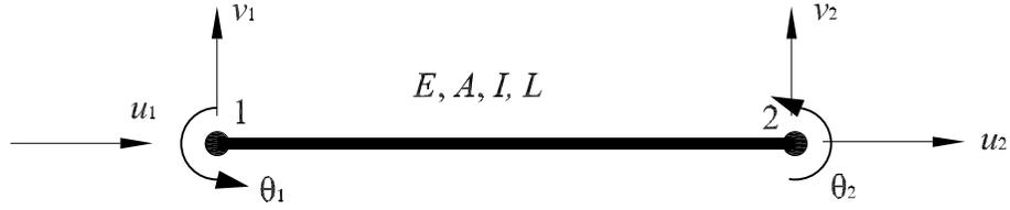
Figure 4.8: A frame element and its nodal d.o.f.
